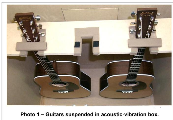
Photo 1 – Guitars suspended in acoustic-vibration box.
