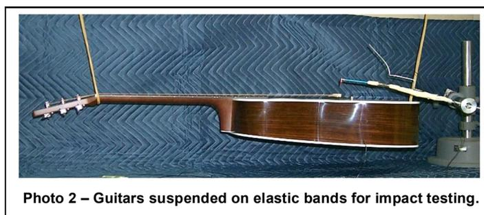
Photo 2 – Guitars suspended on elastic bands for impact testing.
