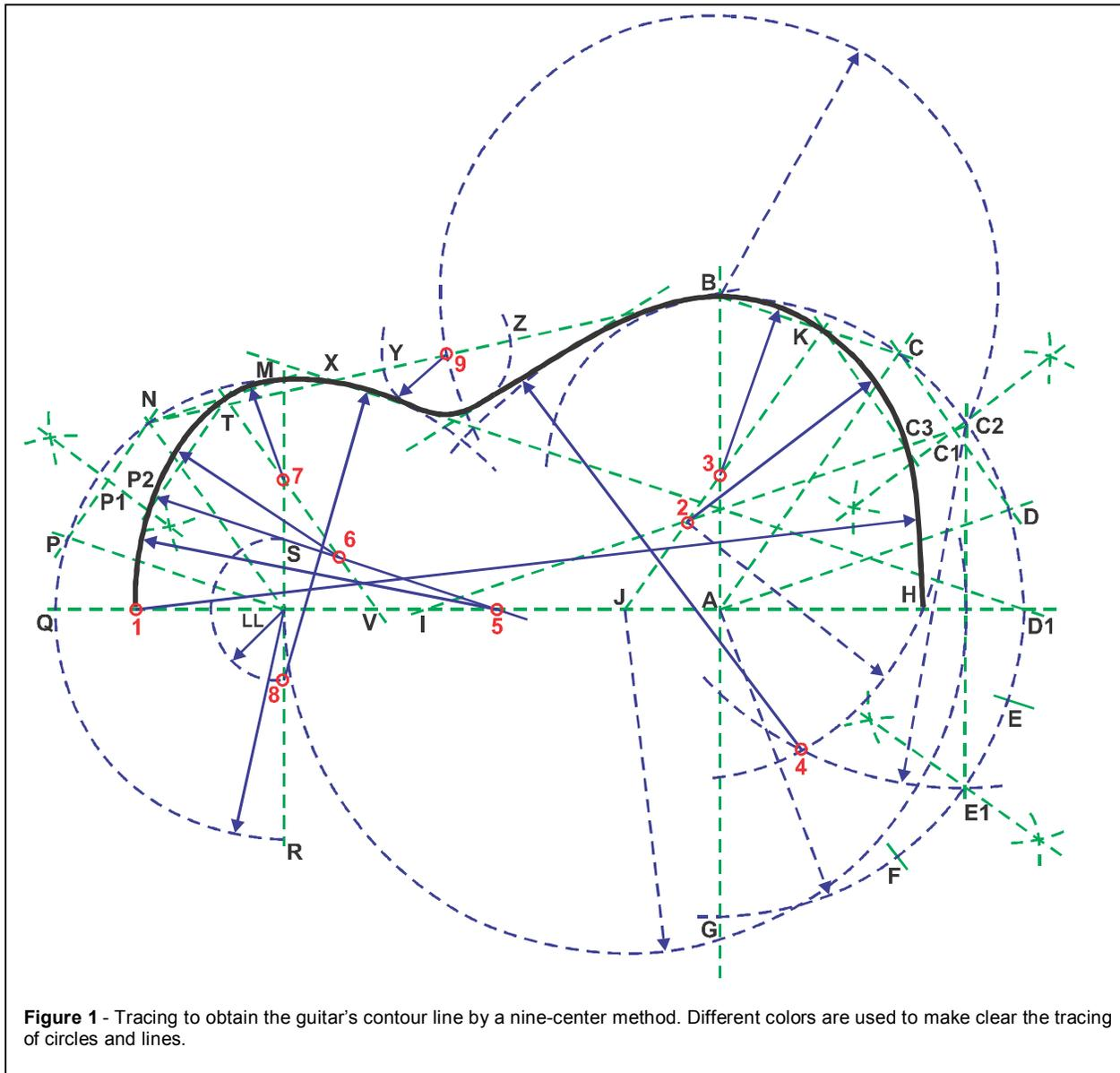
1. A semicircle centered at the initial point A and radius equal to half the lower bout width, is divided in 5 equal parts giving thus points: B, C, D, E, F and G. This can be made with a standard geometrical procedure (for example inscribing a decagon) or with a protractor.
